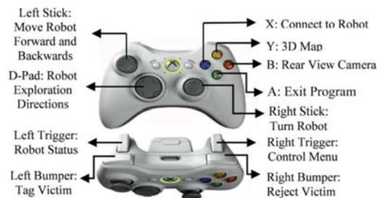
Fig. 15. Xbox 360 wireless controller used as the operator’s input device.
