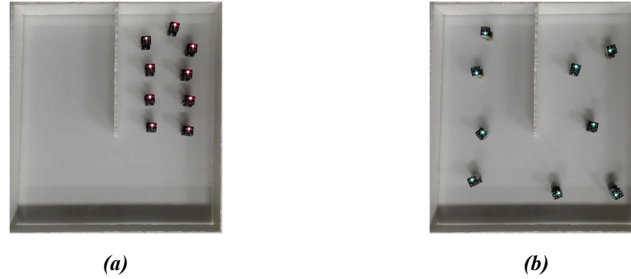
Fig. 9. Second collective exploration behavior experiment demonstrated by mROBerTO s: (a) start and (b) end.
