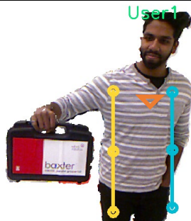
Fig. 7. Tracking Failure example on the right arm (yellow).
