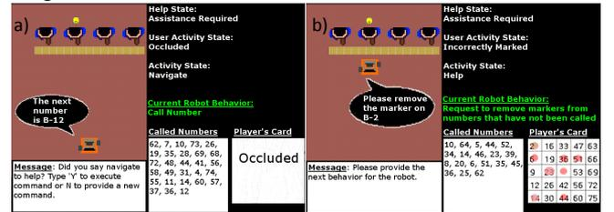
Figure 4. Activity Simulation during a demonstration of a Bingo game: a) robot calls a number and player requests for assistance; b) robot requesting a player to remove marker from uncalled number.
